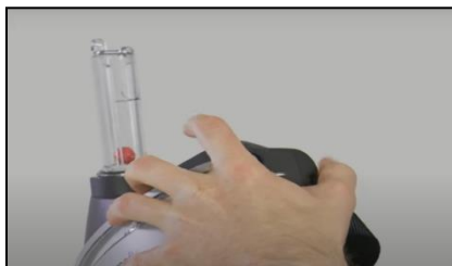
b. Turn ON the PAPR, hold turbo unit and flow meter in a vertical position
