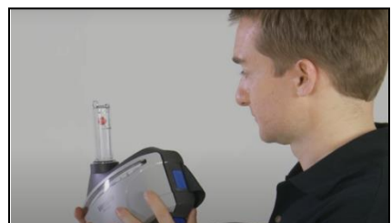
c. Floating ball inside the airflow indicator tube should rise above the appropriate marking level
