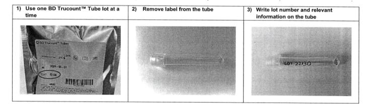
Removal of the label prevents it from interfering with any auto-loading sample preparation and analysis systems, as well as from sticking to other tubes.
